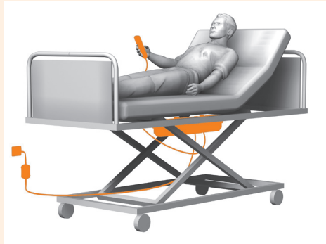
As soon as the hand control is actuated, the actuator is connected to the mains.
